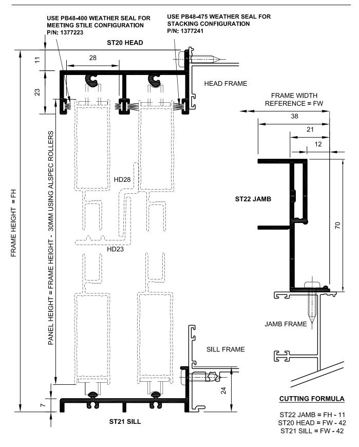
NOTE: FRAME REQUIRES 6G x 1 INCH STAINLESS STEEL PAN HEAD SCREWS
